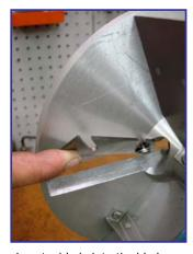
Insert a blade into the blade slot and hook the slot of the blade on the screw closest to the center of the cutter. Swing the blade down into position and insert the 2<sup>nd</sup> screw and washer.
