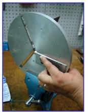
Place the gauge under the edge of the blade. Extend the blade out until the edge can barely be felt when stroking a finger over the blade. Tighten the screws only until snug, just enough to lightly hold the blade in place.
