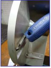
Tap the blade out toward the gauge if the edge cannot be felt when stroking across the gauge.
