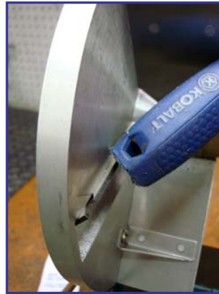
Tap the blade out toward the gauge if the edge cannot be felt when stroking across the gauge.
