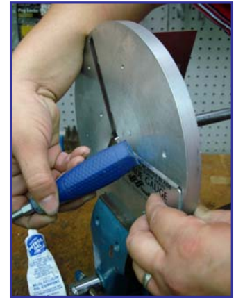
Tap the blade in if too much of the blade edge can be felt. Be certain to use a wooden or plastic handle screwdriver.
