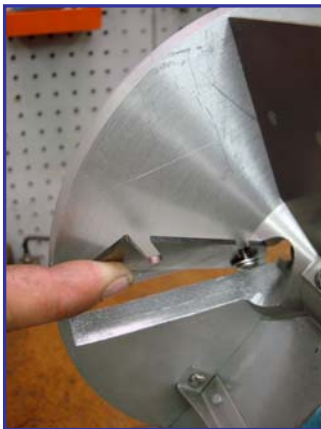
Insert a blade into the blade slot and hook the slot of the blade onto the screw closest to the center of the cutter. Swing the blade down into position and insert the 2 nd screw and washer.
