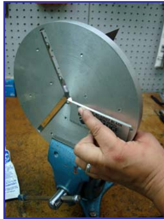
Place the gauge under the edge of the blade. Extend the blade out until the edge can barely be felt when stroking a finger over the blade. Tighten the screws only until snug , just enough to lightly hold the blade in place.
