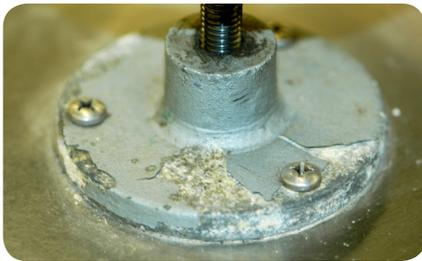
An aluminum flange on a competitor's machine after long-term exposure to stainless steel in a humidity. Even though this metal had been painted, water was still able to penetrate and facilitate galvanic corrosion.
