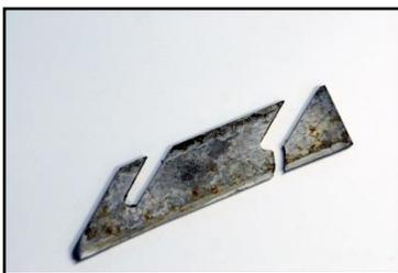
*This blade has cracked as a result of calcium deposits which formed on the underside. Water trapped between the blade and the cutter caused a catalytic reaction to occur. Calcium crystals formed and pushed up against the blade, cracking it at its weakest point; the screw slot.*
