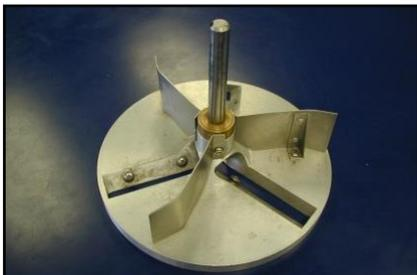
*Cutter shown with 3 bent fins. This occurred at our own SnoWizard® SnoBall Shoppe when the operator inserted an ice pick in the chute to remove clogged snow. Ironically, a water sprayer mounted on the drip pan, specifically for this purpose, was not used by the employee.*
