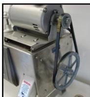
**Let's start the cleaning by removing the belt guard and the cutter assembly.** To remove the belt guard, loosen the four wing nuts that attach it to the cabinet. These should be finger tight only with no tools needed to loosen and remove them. Slip off the belt as you would a bicycle chain off a sprocket.
