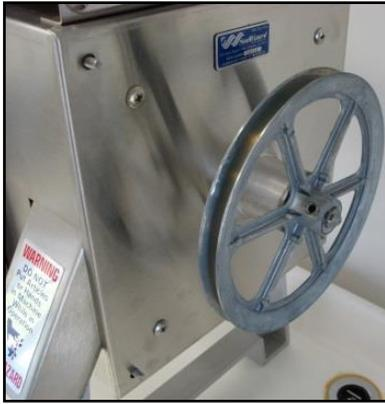
*Place the cutter assembly on the cabinet and hold it in place with one hand. Do not put the wing nuts on.*
