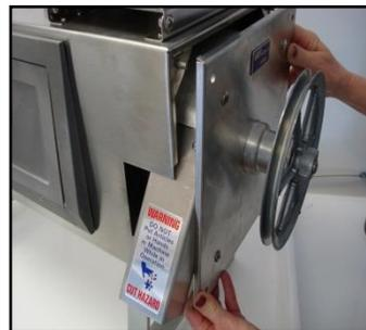
*With the wing nuts and belt removed a firm tug will separate the cutter head from the cabinet. It is not necessary to remove any additional nuts or bolts from the cutter assembly.*
