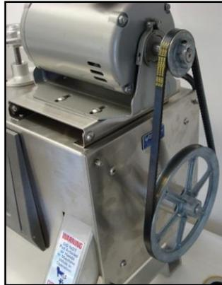
*While holding the cutter assembly to the cabinet, place the V-belt on the small motor pulley and rotate around the large cutter pulley.*
