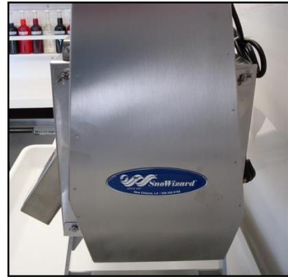
*Next, place the belt and pulley guard on the threaded studs and screw on the four wing nuts. No tools should be used; finger tighten only.*
